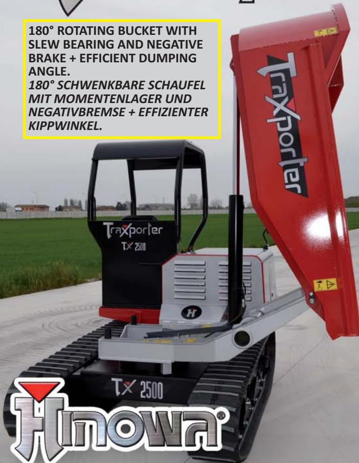
TURNABLE REVERSE OPERATOR SEAT WITH POSSIBILITY TO GET IN-OUT FROM EITHER SIDE.
